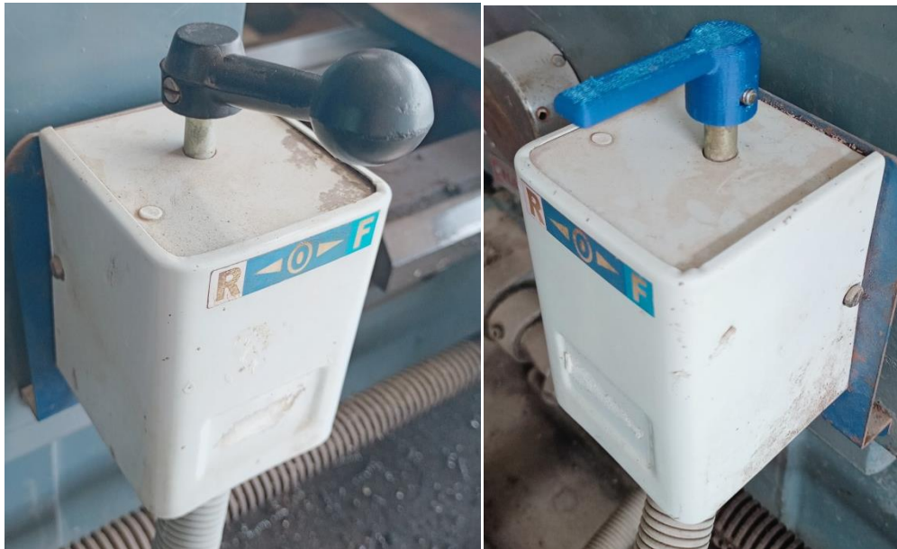
Lathe machine damaged ON/OFF lever is replaced with 3D Printed lever
